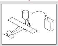
Empty the fuel tank after flying, fuel the tank can cause corrosion and lead to engine problems.
