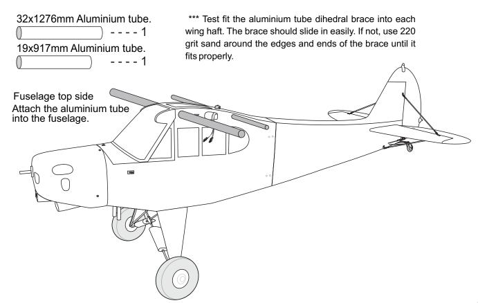
Attach the wings to the joiner tube and secure the wing panels to the fuselage. Main wing must be inserted and attached completely before fixing with screw.
