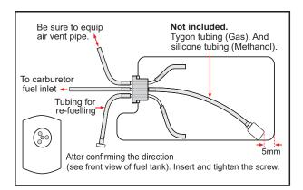
5) Test fit the stopper assembly into the tank. It may be necessary to remove some of the flashing around the tank opening using a modeling knife. If flashing is present, make sure none of it falls into the tank.
