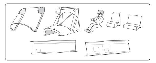
Position the canopy so the rear frame on the canopy is aligned with the rear edge of the cockpit opening. Use canopy glue to secure the canopy to the canopy hatch. Use low-tack tape to hold the canopy in position until the glue fully cures. Wrap the tape completely around the canopy hatch.
