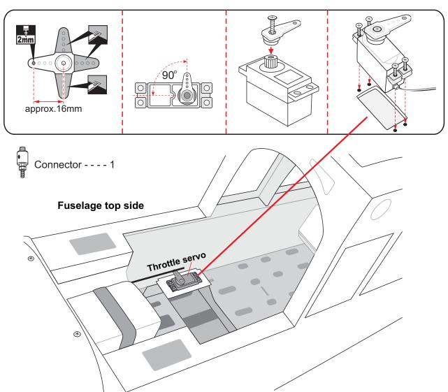
1) Install one adjustable metal connector through the third hole out from the center of one servo arm, enlarge the hole in the servo arm using a 2mm drill bit to accommodate the servo connector. Remove the excess material from the arm.
